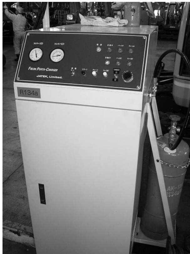
Vacuum and charging unit in the Hirakata Factory Assembly Line.
